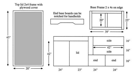
Measure and cut plywood as indicated in drawing above. Cut the 12 foot 2" by 4" into five pieces: two 39", two 23", and one 20" long. Nail the 2" x 4"s together on edge with two 16d nails at each joint as illustrated in the Base Frame diagram. Nail the plywood base piece onto the 2" x 4" frame.
