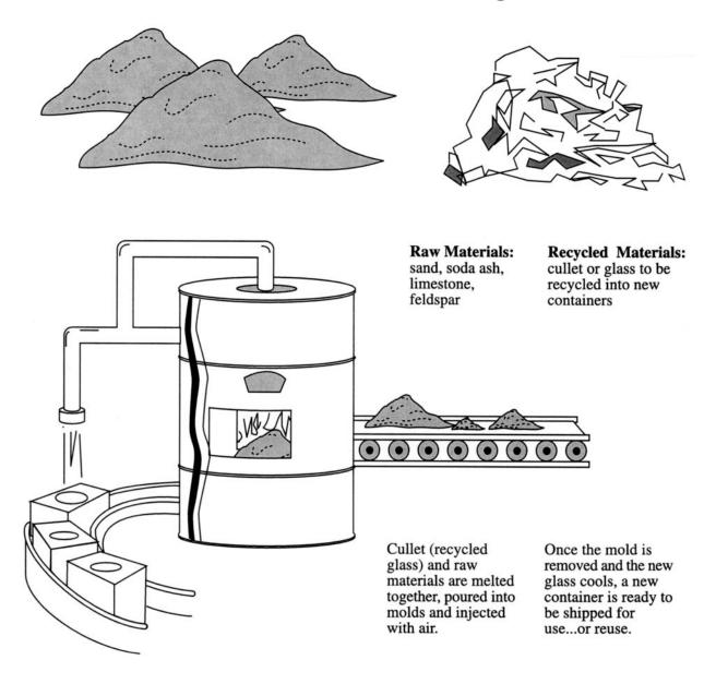
1,330 pounds (603 kg) of sand, 433 pounds (196 kg) of soda ash, 433 pounds (196 kg) of limestone, 151 pounds (68 kg) of feldspar and 15.2 million Btus of energy are required to make just one ton of glass. Major deposits of white sand suitable for making glass are found in Illinois, New Jersey, the Alleghenies and the Mississippi Valley. Most soda ash comes from Wyoming, and 65 percent of the feldspar in the United States comes from California and North Carolina.
